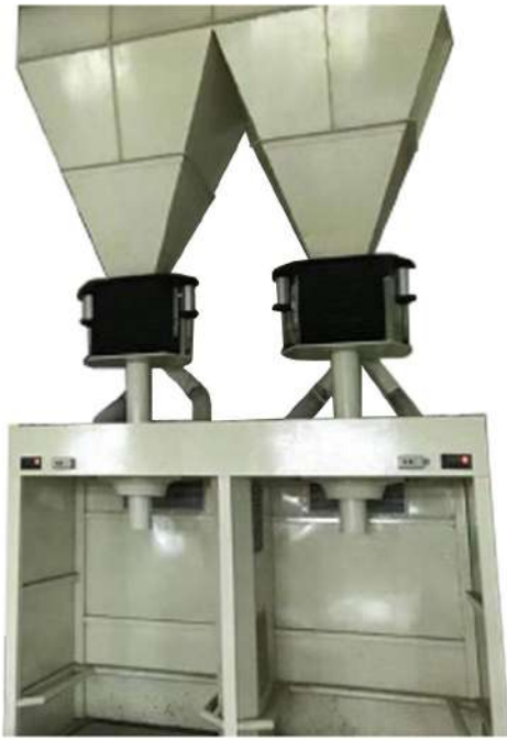
Powder receiving station 接粉站
