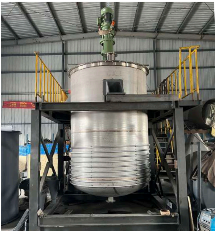
Aging Tank 老化罐
